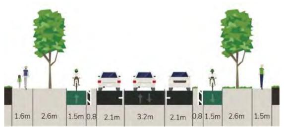
Figure 15: Conceptual cross-section of potential amended bike lane with intermitted raised separator and painted lines for Kent Road, Pascoe Vale between Cornwall Road and Cumberland Road.
