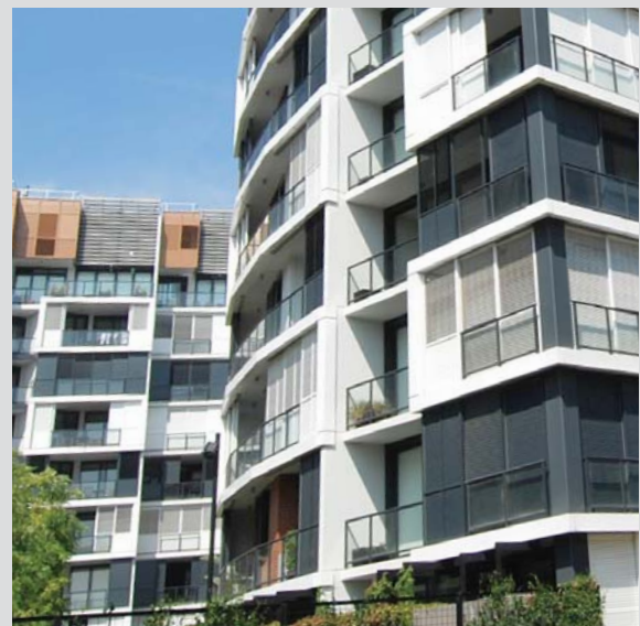
2.6.6 Flexible sliding louvred screens provide privacy to suit building occupants and create a dynamic facade
