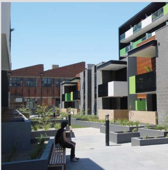
2.6.5 Solid balustrades on the lower floors provide privacy for residents with upper level balconies which are not directly visible from the street can have transparent balustrades
