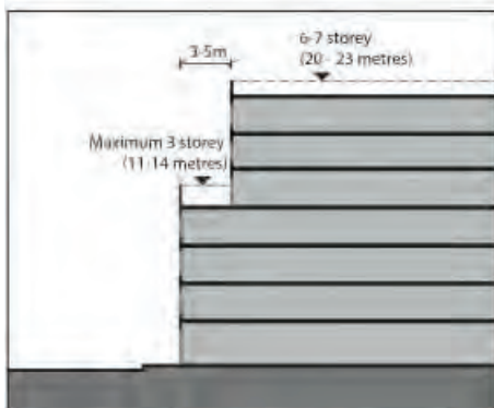
TYPE 4: Maximum 4 storey (11-14 metres) street wall height 3-5 m minimum upper setback
