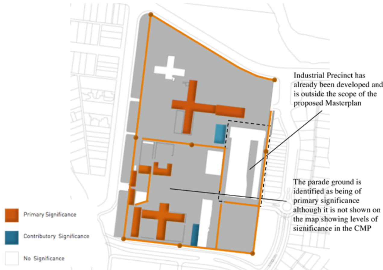
Figure 3 Levels of significance of existing building from the Pentridge Prison CMP
