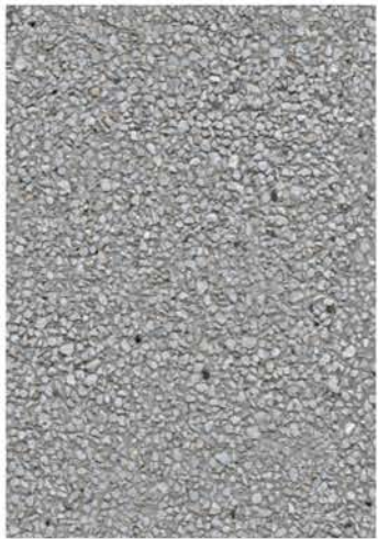
EF-02 EXPOSED AGGREGATE PRECAST
