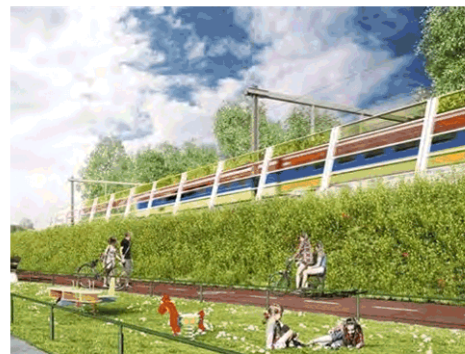
QB44 A2 Highway, Netherlands [Illustration] Luminescent solar concentrators (LSC) and soft landscaping as noise barrier
