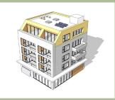
This model should include the external building envelope and any significant projecting structures for detailed shadow analysis purposes. This can include basic colours & material detailing, but it is not required.
