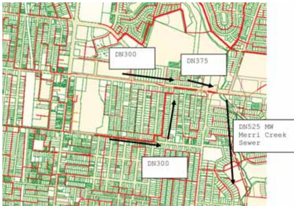
Fig. 2 – Sewer Main flow directions.
