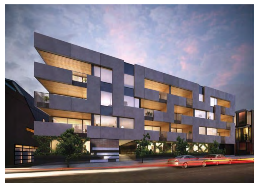
example of creation of recessed balcony space to provide depth and articulation to a facade
