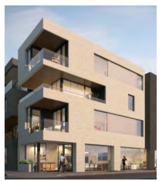
example of creation of recessed balcony space to provide depth and articulation to a facade
